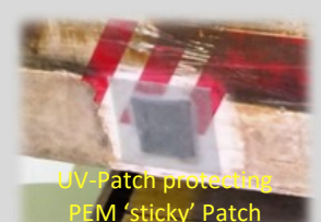
A rupture of a boat Hull use PEM 'sticky' Patch and UV Patch as impact protection to achieve a permanent repair solution. Once fully hard UV- Patch can be used above or below the waterline
