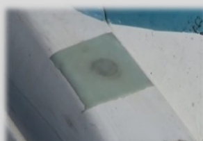
Firmly smooth the entire UV Patch to the damage area. Expose to daylight to fully harden
