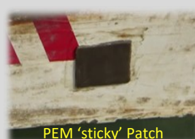
A rupture of a boat Hull use PEM 'sticky' Patch and UV Patch as impact protection to achieve a permanent repair solution. Once fully hard UV- Patch can be used above or below the waterline
