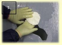
A Hole Sealer Plug expanding through the hull rupture. Note the hand of the applicator compressing the putty on the other side of the semi transparent boat hull structure Massaging the putty in the plastic bag partly filled with water causes the putty to rapidly expand and harden.
