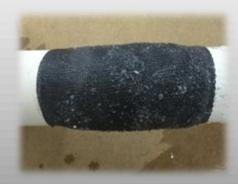
Black Tape as a wrapping reinforcing material is very useful in wetted or saturated repair applications and for general reinforcement to other types o (2)-3ials. air
