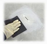
Massaging the Hole Sealer Plug Putty in water will commence a reaction, keep kneading the putty
